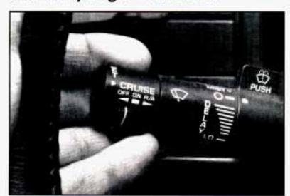
To change the headlamps from low beam to high or high to low, pull the turn signal lever all the way toward you. Then release it.
